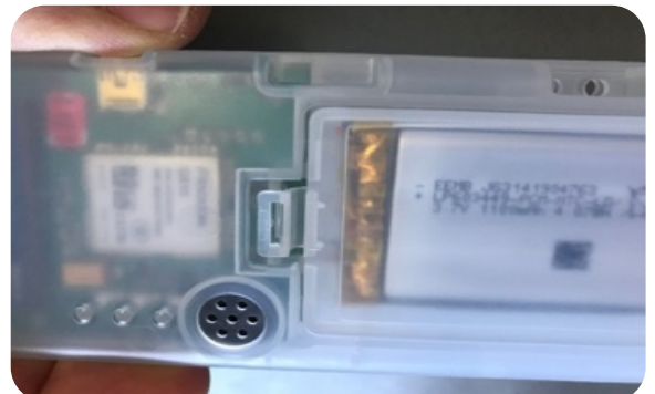
Step 6. Close the back cover, insert the battery and close the battery bay door.
