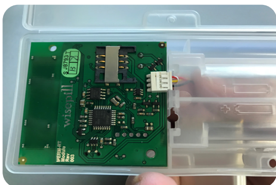
Step 5. Ensure that the battery connector is securely connected, as shown above.
