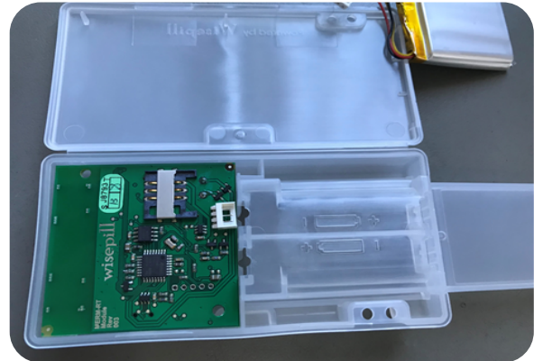
Step 2. Position the module so that the battery connector is exposed
