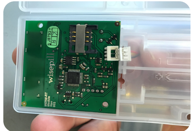
Step 4. Feed the battery connector through the hole in the battery bay, as shown above.
