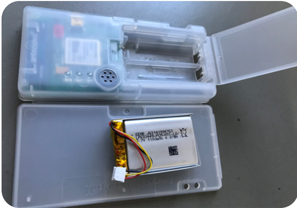
Step 1. Open the battery bay door and back cover and remove the battery
